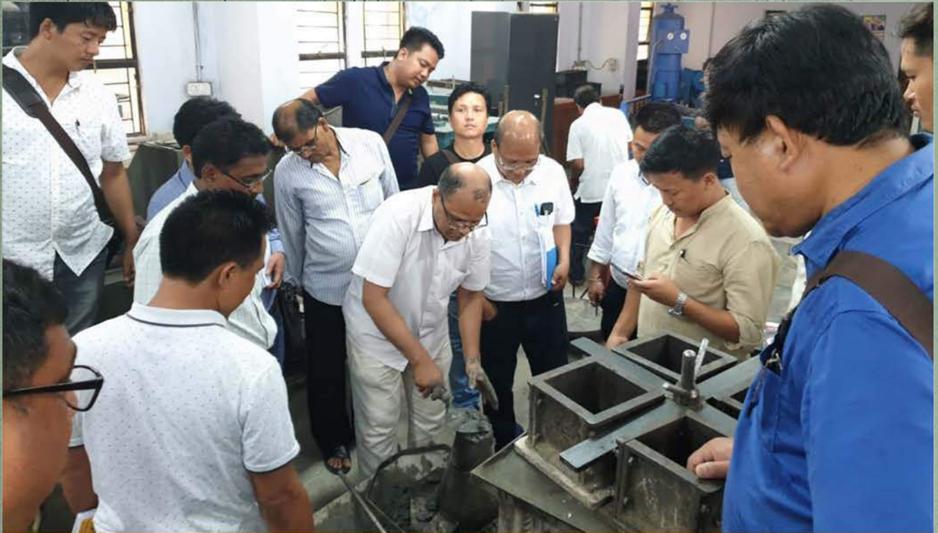
During training in NERIST on Quality Control & Mix Design of Concrete-1st Batch (29th to 30th June 2019) (Casting of cube samples)
