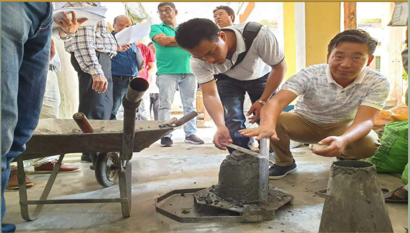
During training in NERIST on Quality Control & Mix Design of Concrete-1st Batch (29th to 30th June 2019) (Performing Slump test)
